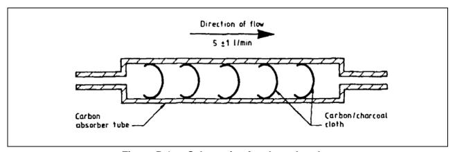
Figure B.1 — Schematic of carbon absorber
